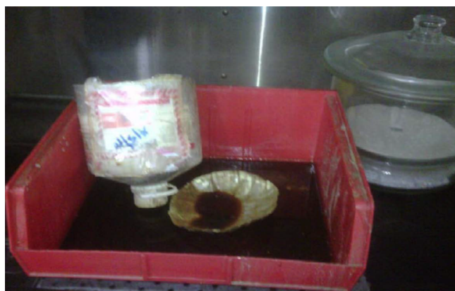
Figure 1. Ruptured waste container and spilled corrosive waste.
