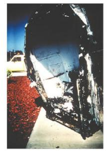
This picture shows a UCI lab refrigerator which exploded when chemicals were inappropriately stored in a unit which was not designed for flammables storage.
