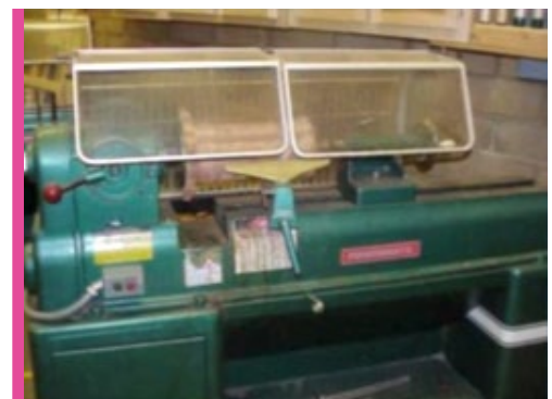
Wood lathe with guards in place.
