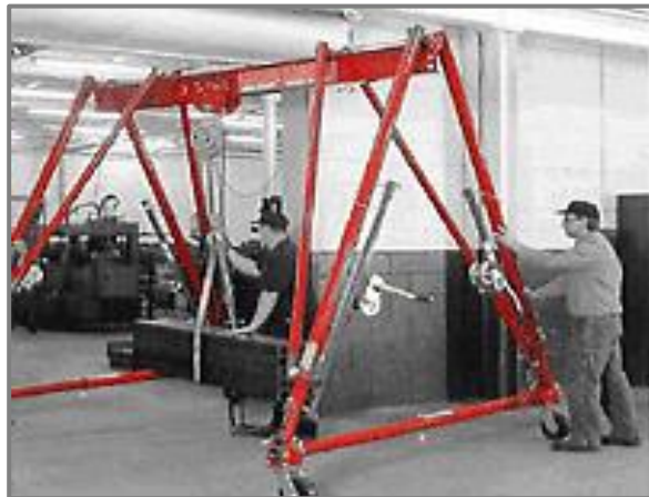
Mobile Gantry Crane
