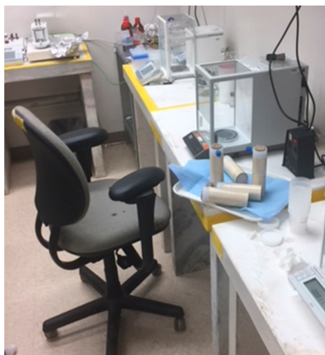
Figure 1. Post-incident photo of the spill area. Unsecured vessels were transferred using an insufficient secondary containment (similar to a lunch tray) which was incapable of containing a spill. Discoloration on the chair is due to acid damage.
