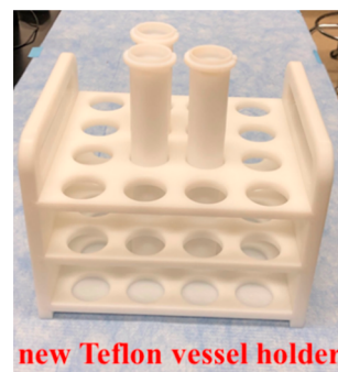
Figure 2. Specially designed Teflon microwave vessel holder. The weight and shape of the holder decrease tipping hazards.
