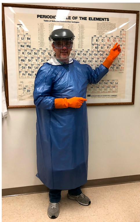
Figure 3. Demonstration of essential PPE required for protection from HF spills. These include close-toed shoes, long pants, vapor protecting chemical splash goggles, plastic apron with full-length sleeves and upper chest protection, face shield with chin splash protection, and nitrile gloves under HF-resistant gloves (Trionic O-240).
