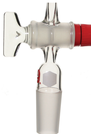
Fig. 5. Septum inlet adapter
