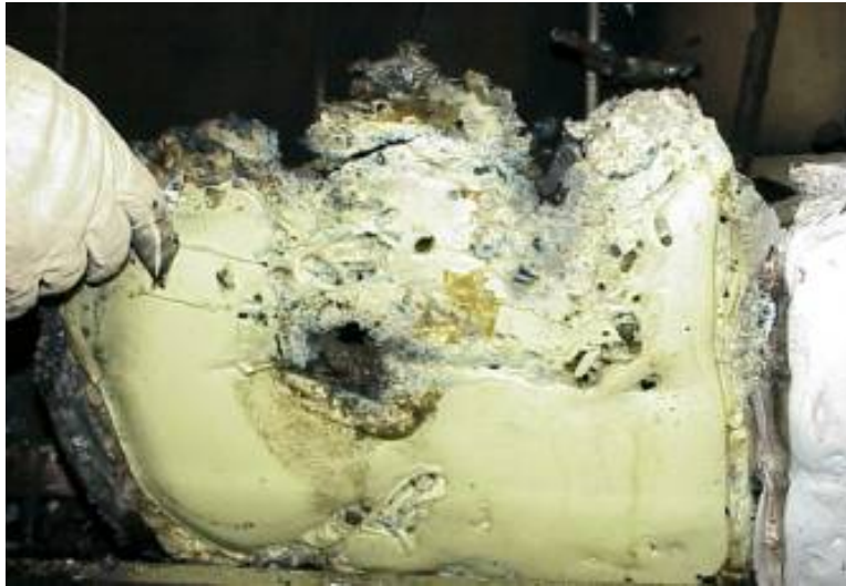
Photo 4. Crater in the bottom of a plastic spill tray, produced by a squeeze bottle containing heated hexane.
