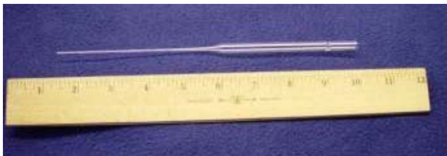
Photo 2. Example of a 2 ml pipette.
