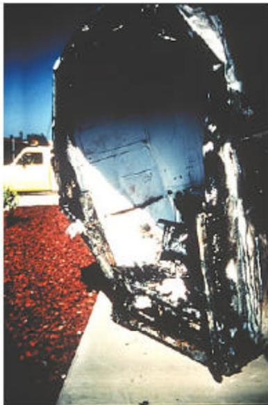
This picture shows a UCI lab refrigerator which exploded when chemicals were inappropriately stored in a unit which was not designed for flammables storage.
