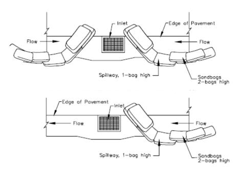
Figure 2 Gravel Bag Barrier for Curb Stormdrain Inlets
