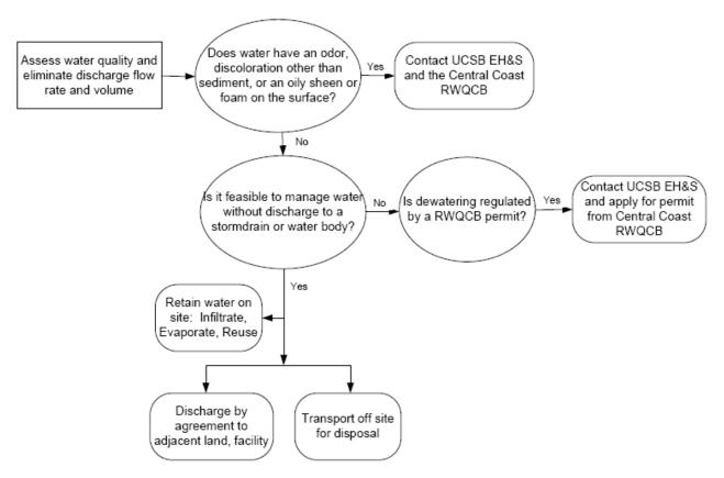
Figure 1 Dewatering Flowchart
