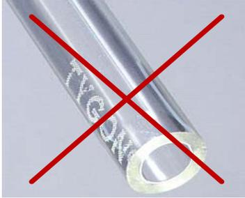
Tygon tubing **should never be used in a closed or pressurized system** regardless of the median or a system where a valve could be closed isolating the tubing to the pressure source. **If used with water it will burst in the future.**
