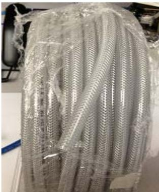
**Acceptable for** use with Inert gases, compressed air, lab water, house vacuum.
