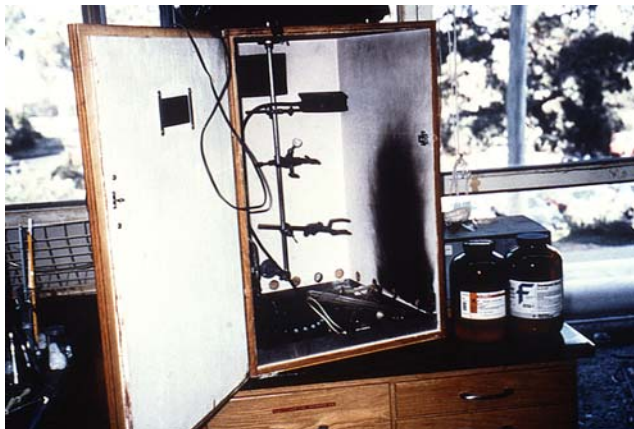
Unlabeled wooden UV-photolysis box showing evidence of fire.
