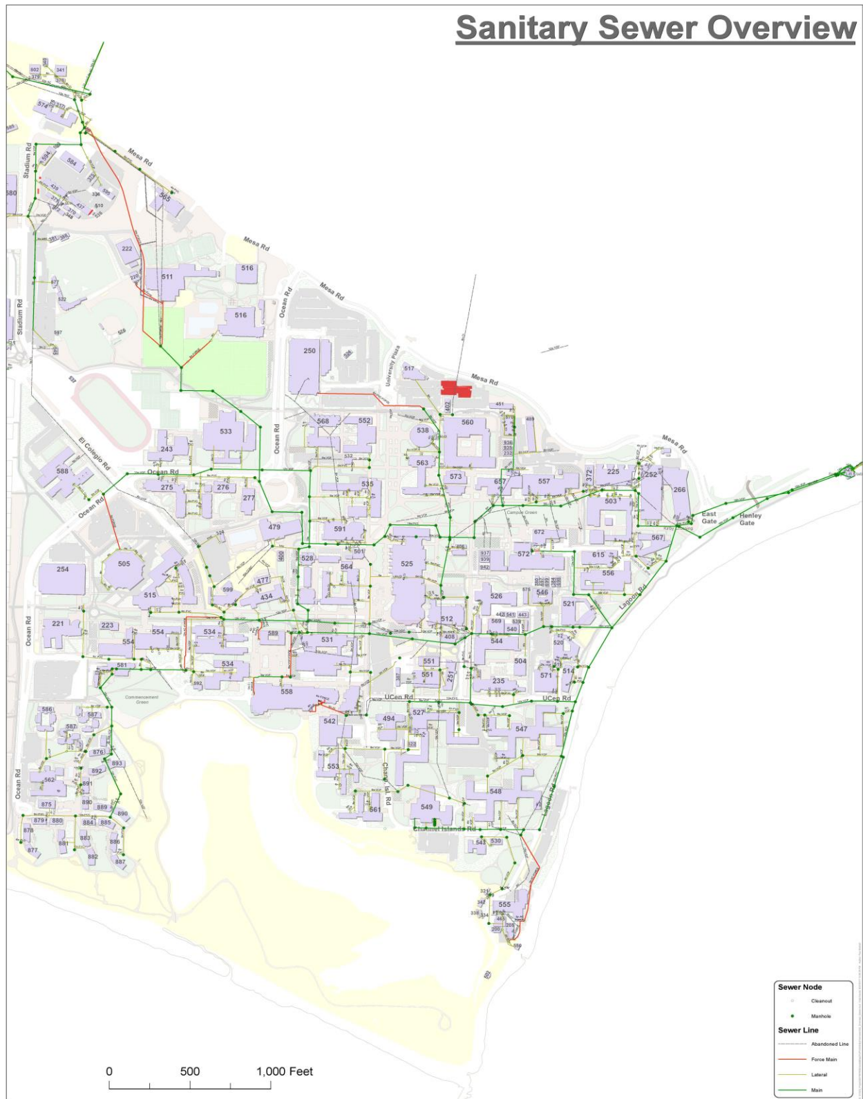
Figure 2-2 UCSB Sanitary Sewer System Map - Main Campus
