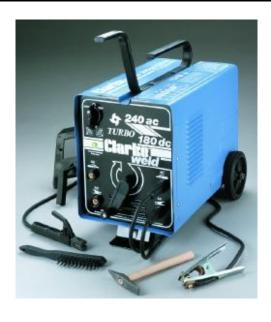
Arc welding is a type of welding that uses a welding power supply to create an electric arc between an electrode and the base material to melt the metals at the welding point.
