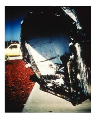
Remains of lab refrigerator after explosion due to inappropriate storage of flammable liquids in normal ("nondesparked") unit.
